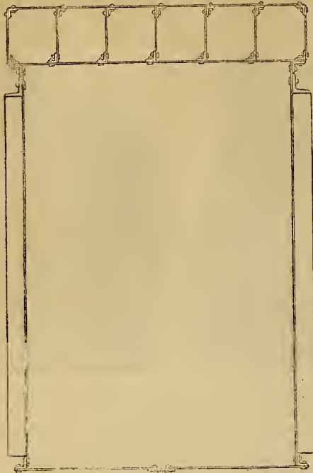
MODEL OF STEPHENSON'S BRIDGE. Transverse Section. Scale, three-quarters of an inch=1 foot.
